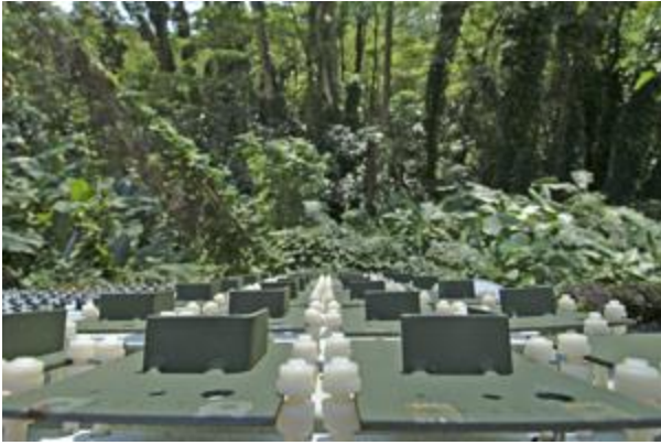
An Army test yard at Lyon Arboretum in Hawaii tests for corrosion in the rainforest microclimate. Photo by Ryan Sugamoto, University of Hawaii.
