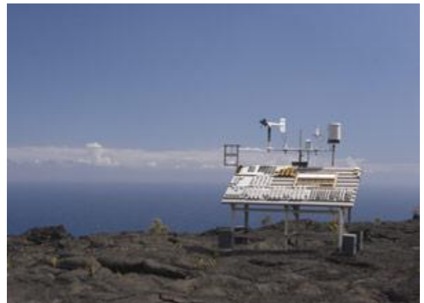
A test yard at Volcanoes National Park in Hawaii tests for corrosion in the volcanic microclimate. Photo by Ryan Sugamoto, University of Hawaii.
