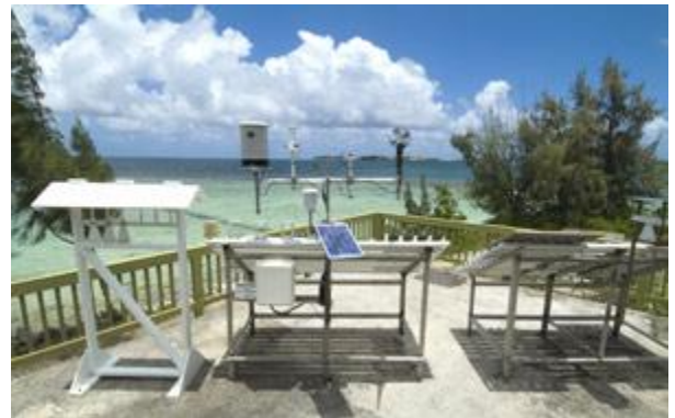
The Army's Pacific Rim-based corrosion testing takes place in a tropical marine microclimate. Pictured is a corrosion test yard on Coconut Island, Hawaii. Photo by Ryan Sugamoto, University of Hawaii.
