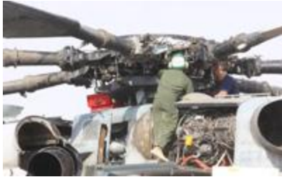
A U.S. Marine, left, and a civilian contractor with Marine Heavy Helicopter Squadron 465, work on the gearbox of an H-53 helicopter in Al Asad, Iraq, in the fall of 2006. Photo by Cpl. Richard A. Hilario, U.S. Marine Corps.
